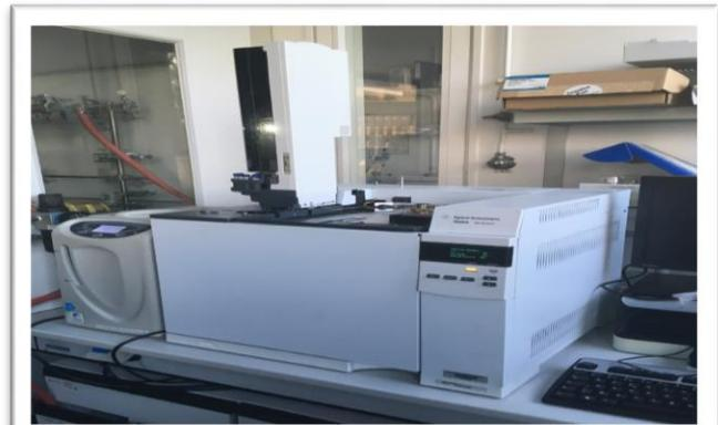
Picture 4 : The GC-FID system (Agilent®)
